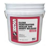
Southcrete 901 Clear Penetrating Sealer is a non-flammable, no-sheen, stain-resistant, water-based penetrating sealer that may be used over all natural stone any other unglazed porous surface where a natural look is desired. Clear Penetrating Sealer permits vapor transmission and for new installations, clear penetrating sealer can be applied 48 hours after grouting.
